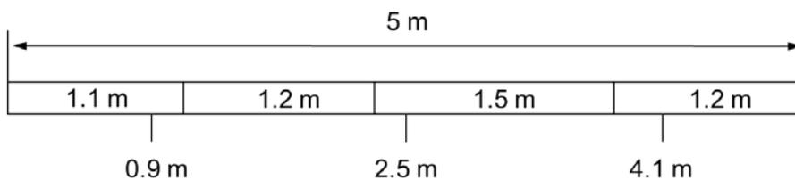
Figure 12: Length of the exhaust air openings
