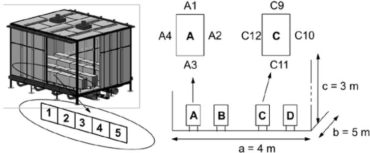
Figure 6: Geometry information of the heat sources
