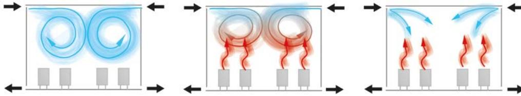
Figure 2: Air flow structures (supply air from both sides), left: isothermal, center: mixed convection wherein the forced convection is dominant, right: mixed convection, wherein neither of the two forces is dominant
