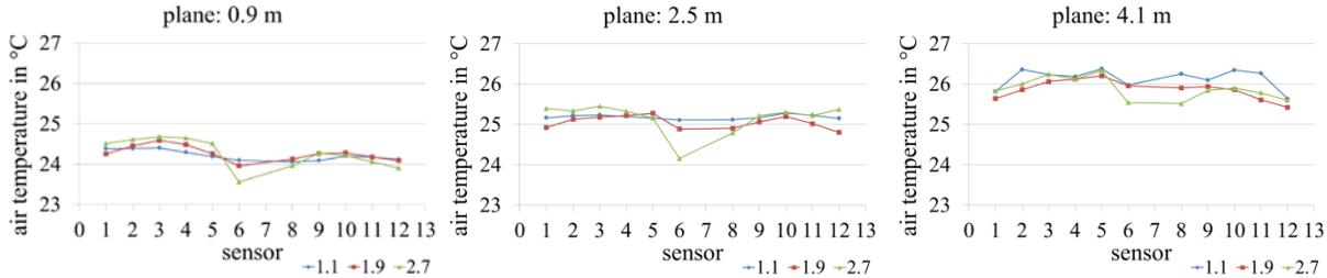
Figure 9: Mean values of the room air temperature in the model room for three measurement planes at inlet velocities of 1.5 m/s and thermal loads of 2 kW
