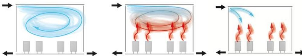
Figure 3: Air flow structures (supply air from one side), left: isothermal, center: mixed convection wherein the forced convection is dominant, right: mixed convection, wherein neither of the two forces is dominant
