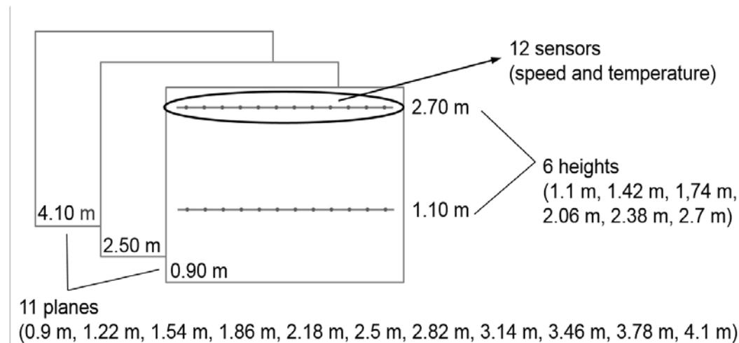
Figure 4: Measurement planes and heights in the Aachen model room
