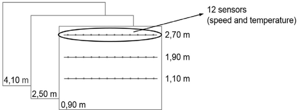
Figure 5: Measurement planes and heights for the simplified presentation of the results
