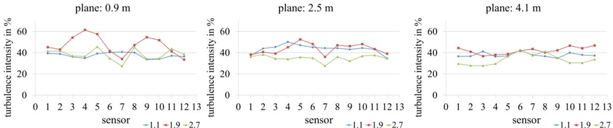
Figure 8: Mean values of the turbulence intensities in the model room for three measurement planes at inlet velocities of 1.5 m/s and thermal loads of 2 kW
